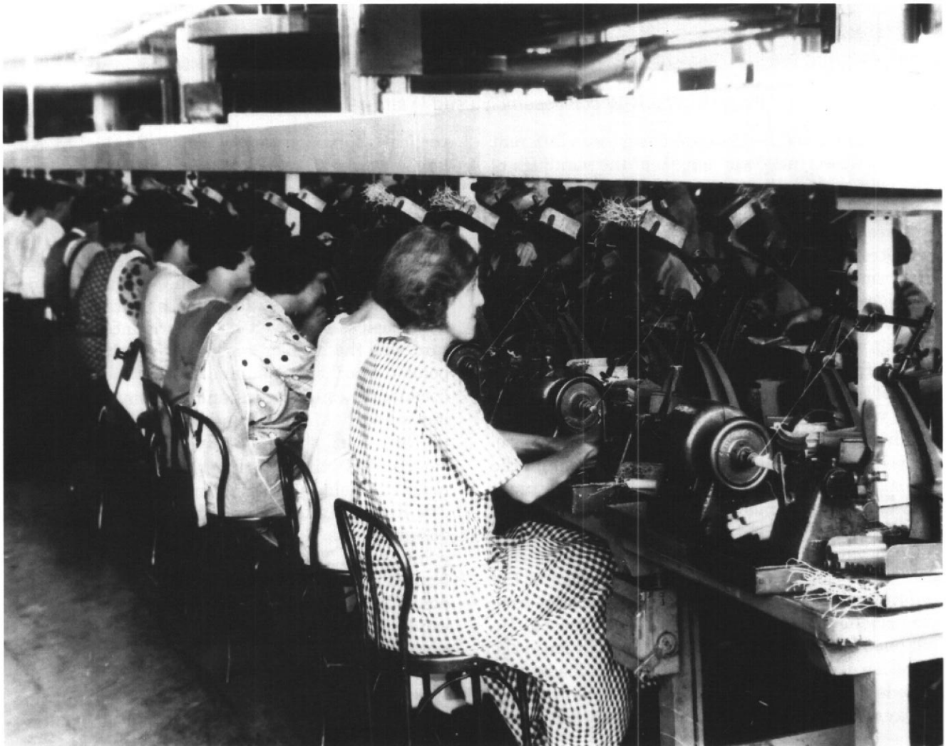
Photo 12: (Bottom Right Facing Page) The photograph shows the final assembly of the coil units. Empty boxes can be seen on the left, and as they progress towards the right hand side of the picture, the various components of the coil are being added.
